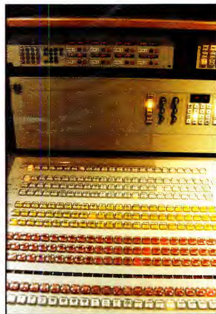
Identical switchers in control room A and B have a router mounted above that can call up any of the 128 sources in house and assign them to eight positions on the switcher. (See eight LED readouts at upper left of photo.)
