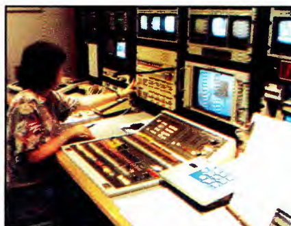
WFTV master control has a router panel with keypad where the operator can call up any of the 128 sources in the house and assign any eight to the small switcher. LED readouts in black windows in the center of the switcher indicate sources assigned.
