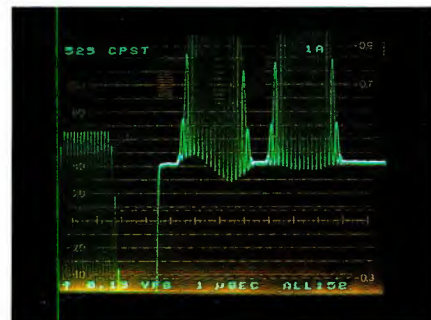
Figure 2. Dual timing pulses indicate a slight gain equality in the Y/R-Y channel, and a timing delay in the Y/B-Y channel.
